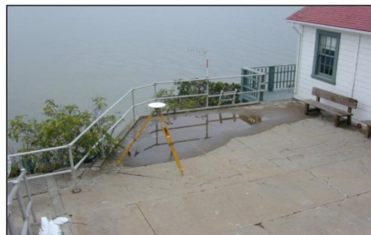
RTK Reference Station on Yerba Buena Island
